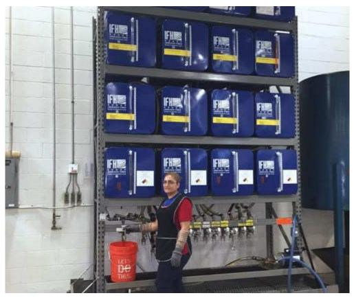
Replacing the outdated 55-gallon drum method with a storage and dispensing system from The IFH Group has made DuPage's oil room operation cleaner and more efficient, with considerable space savings.
