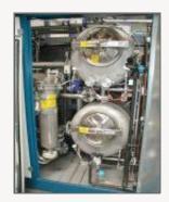
An inside view of the machine cabinet shows the simple organization of the components, providing easy access for maintenance. Large doors in the back of the cabinet also contribute to accessibility. Here are the two fully enclosed flood tanks.
